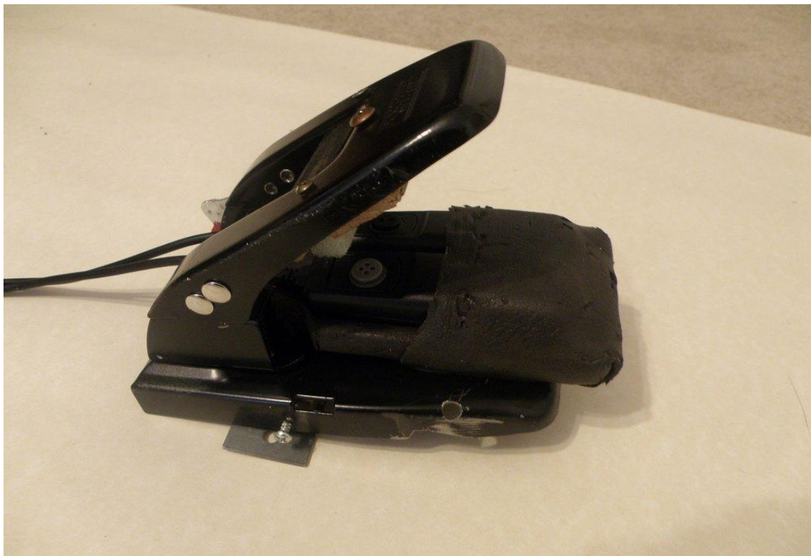
My new dual remote shutter control, made from a two hole paper punch.
