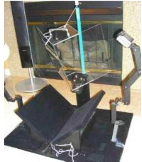
Just one of the many similar designs which utilizes dual trays to secure and image books.
