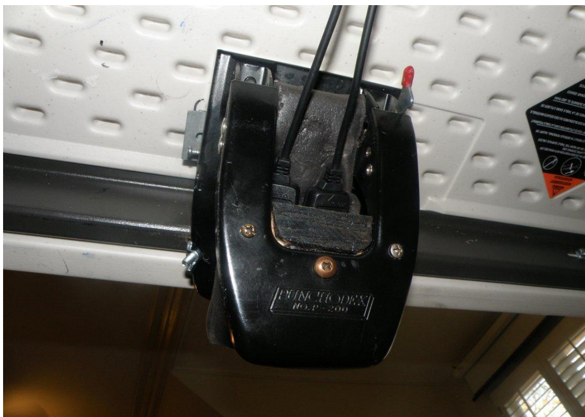
New dual remote shutter control mounted under the table and activated by a knee bump. It would work 56,000+ times, without a hitch.
