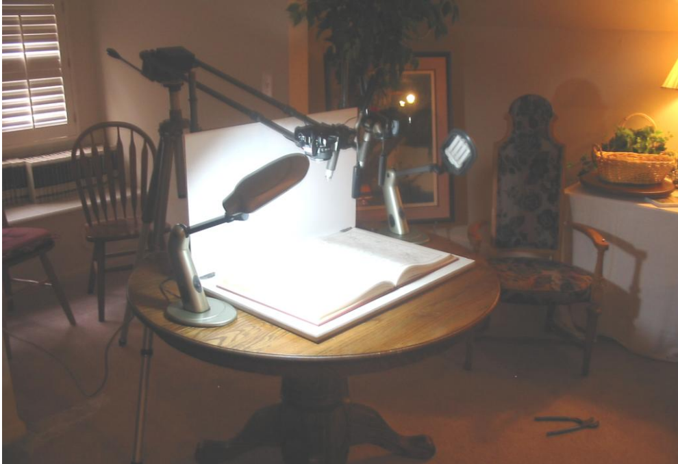
First tripod set-up with extensions created from 1/2 inch water pipes.
